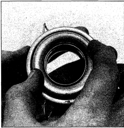
4.4 To check the operation of the bearing, hold it by the outer race and rotate the inner race while applying pressure - the bearing should turn smoothly - if it doesn't, replace it
