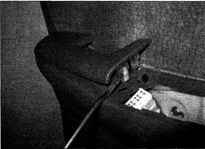
11.5a Pry the armrest up with a screwdriver or trim tool . . .
