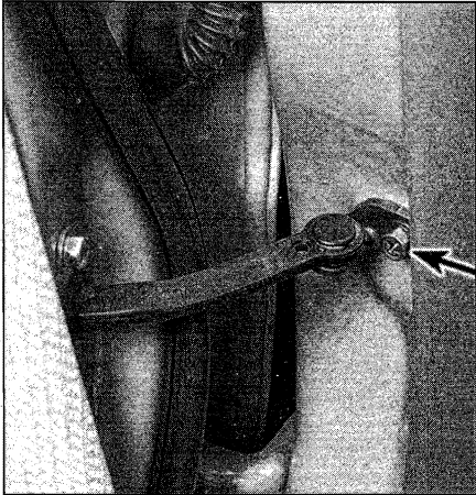
12.3 Remove the bolt and detach the stop strut
