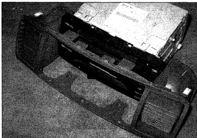
12.3 The radio comes out with this panel and two vents - release the clips top and bottom to remove the radio from the vent panel
