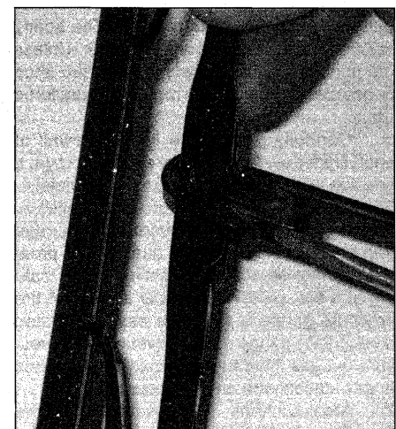
7.5 Push on the release lever and slide the wiper assembly down out of the hook in the end of the wiper arm
