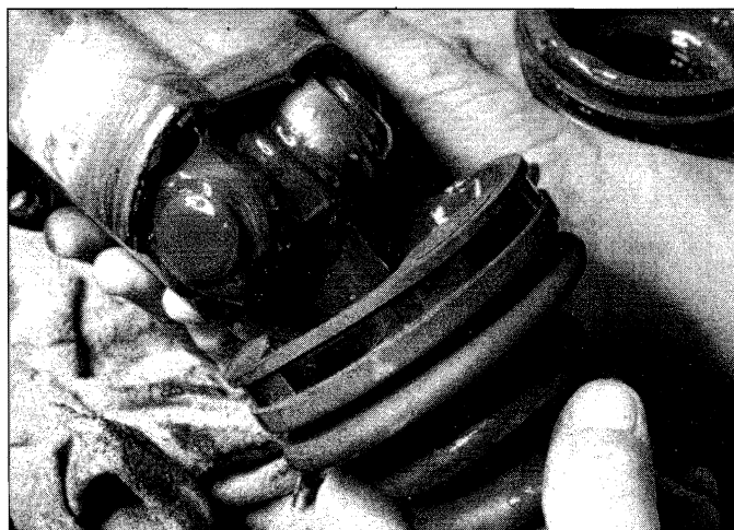
11.4 Remove the boot from the inner CV joint and slide the joint housing from the tripod
