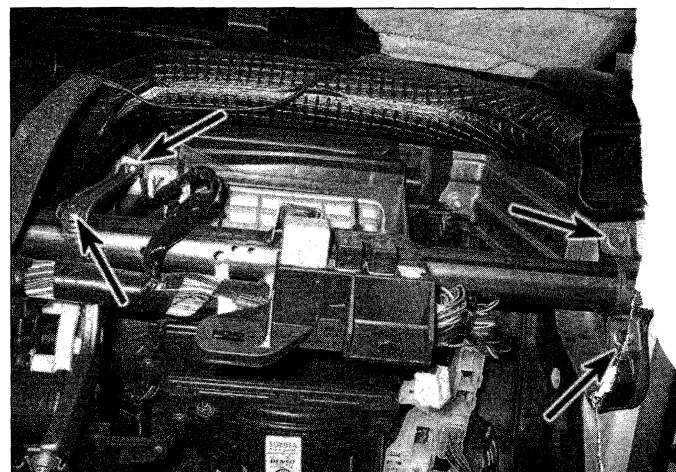
10.8b The cross-cowl support tube is secured to the vehicle at each side - remove the bolts and clamp at each end (right side shown)
