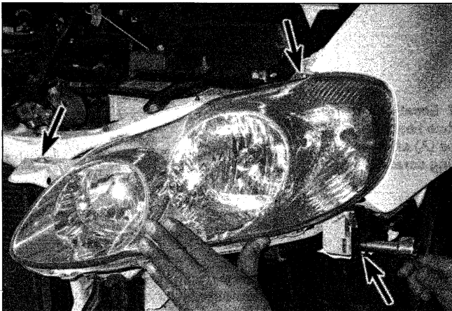
17.2 Headlight housing mounting screws
