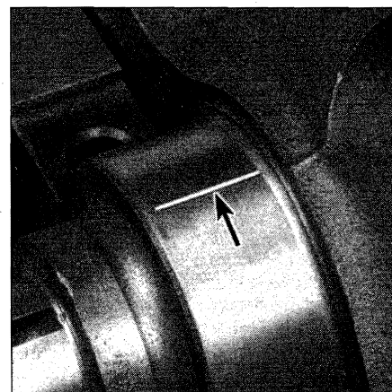
10.17 Place the Plastigage onto the crankshaft bearing journal as shown
