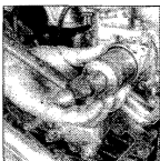
9.7b As a last resort, you can also drive a seal into place with a hammer and a large socket, but make sure you don't damage the sprocket positioning pin on the end of the camshaft
