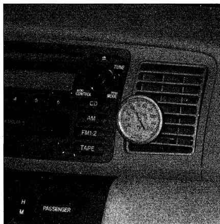
12.10 Check the temperature of the output air in the center register with a thermometer - it should be 35-40 degrees below the ambient air temperature
