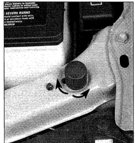
9.11 Adjust the hood height by screwing the hood bumpers in-or-out
