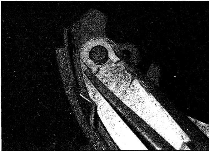
6.4m Assemble the parking brake lever to the new rear shoe and crimp the C-washer closed with a pair of pliers (always use a new C-washer)
