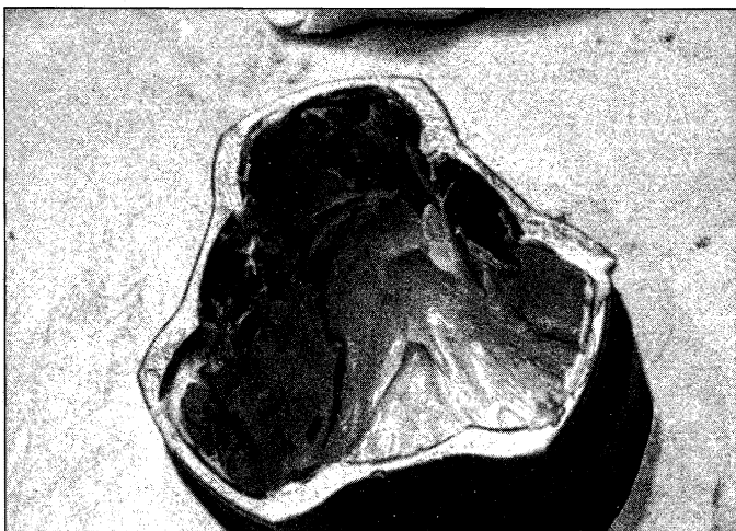
11.10b Place grease at the bottom of the CV joint housing
