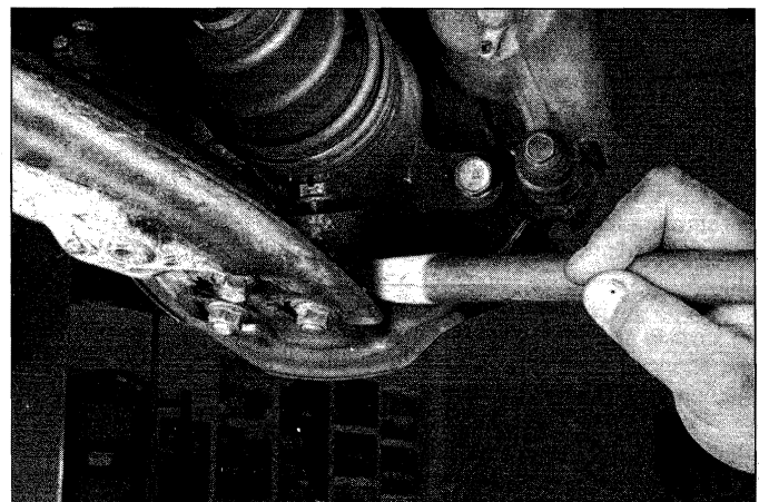
6.3 Separate the balljoint from the steering knuckle with a picklefork-type balljoint separator
