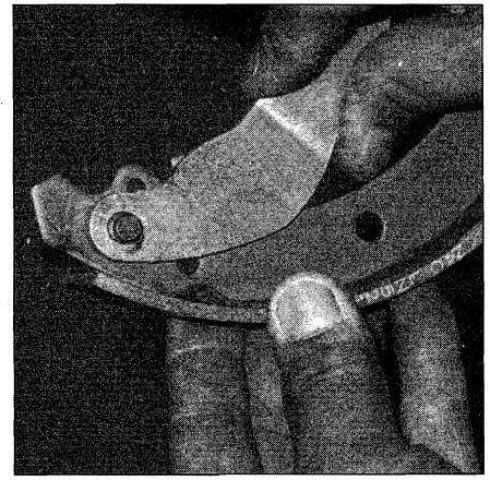
6.4l Remove the parking brake lever from the rear shoe
