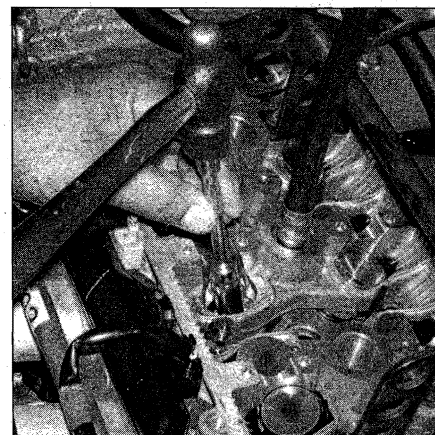
6.15 Using a deep socket and hammer, gently tap the new seals onto the valve guide only until seated
