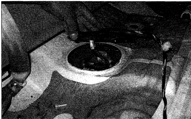
5.4 On 2003 and 2004 models, pry the fuel pump access cover off (it's secured by butyl tape). On 2005 models it's secured by four screws
